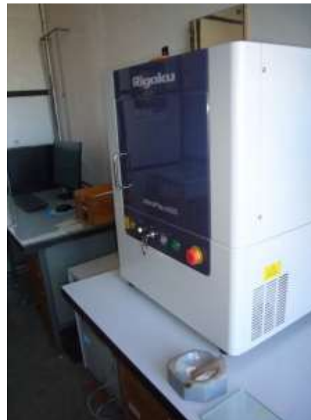
RTG difraktometer RIGAKU MiniFlex600, Theta-2Theta, \text{CuK}\alpha
